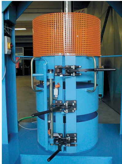
Three-Section Steel Jacket with Toggle Catch
