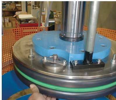
Double O-Ring with Vent Valve
